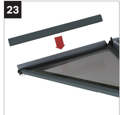
23 Work your way around the roof and fit the rafter top caps. Fitters tip: Suggested top cap installation order is hip top caps followed by the ridge top cap and finally any rafter top caps.
